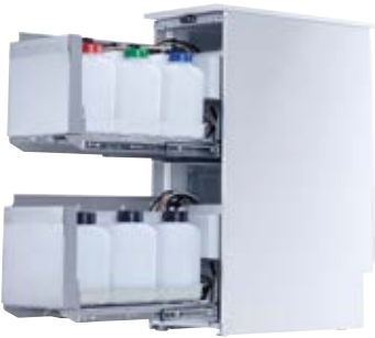
PG 8596 Dispensing unit, for detergents and dispensing modules, white. • 2 removable drawers for 3 x 5 l canisters each • Interior dimensions: H 285–690, W 250, D 425–555 mm • 2 loading options per level for dispensing modules • Drip tray facilitates better residual emptying of canisters • H 835, W 300, D 600 mm
