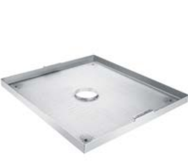
E 319/4 Surface filter, for optimum protection against contamination from labels or glass splinters. • Surface filter for coarse soil • Filters out laboratory glassware labels • Prevents contamination with splinters of broken glass • For use in all PG 85 undercounter laboratory washers • H 39, W 455, D 513 mm
