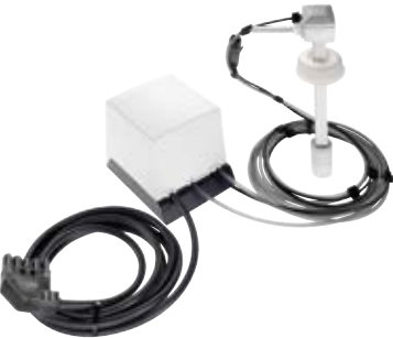
DOS K 85/1 Comfort Dispensing module for 5 l canisters, for automatic dispensing of liquid media, with fill level detection. • Dispenser monitoring – high process security as per EN ISO 15883 • Permanent monitoring of the fill level and integration option in Miele MOVE to create customised notifications • For dispensing liquid cleaning agent/neutralising agent • 214 mm suction lance for 5 l media canisters with flexible cap • Suction lance conversion kit for 10–30 l canisters available from Customer Service
