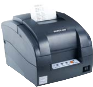
APH 510 PRT 110 Report printer for process protocols. • Dot matrix printer with ink ribbon • Compatible with Miele PG 8583, PG 8593, PG 8583 CD and PLW 6x11 laboratory washers • H 157, W 160, D 239 mm
