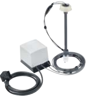
DOS K 85 Flex Dispensing module for 5–10 l canisters, for automatic dispensing of liquid media, with “container empty” monitoring. • Dispenser monitoring – high process security as per EN ISO 15883 • For dispensing liquid cleaning agent/neutralising agent • 352 mm suction lance for 5–10 l canisters, with flexible cap • Suction lance conversion kit for 10–30 l canisters available from Customer Service
