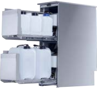
PG 8596 Dispensing unit, for detergents and dispensing modules, stainless steel. • 2 removable drawers for 3 x 5 l canisters each • Interior dimensions: H 285–690, W 250, D 425–555 mm • 2 loading options per level for dispensing modules • Drip tray facilitates better residual emptying of canisters • H 835, W 300, D 600 mm
