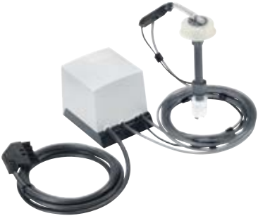
DOS K 85/1 Flex Dispensing module for 5 l canisters, for automatic dispensing of liquid media, with “container empty” monitoring. • Dispenser monitoring – high process security as per EN ISO 15883 • For dispensing liquid cleaning agent/neutralising agent • 214 mm suction lance for 5 l media canisters with flexible cap • Suction lance conversion kit for 10–30 l canisters available from Customer Service
