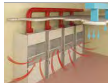
Automatic microprocessor control of the air intake and compensation system for a laboratory with one or more hoods.
