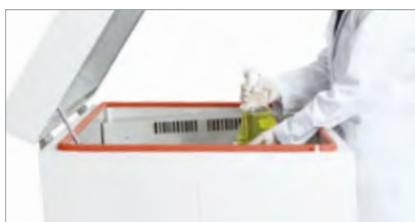
Easy to attach and detach large-volume sample (ISF) thanks to the inclined structure. (registered design 30-2014-0060254)
