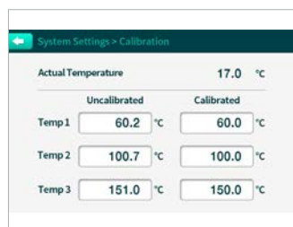
Accurate temperature control with 3-point calibration
